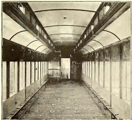
CONSTRUCTION VIEWS TAKEN DURING APPLICATION OF HEAT INSULATION AND AFTER THAT OF WAINSCOTING AND STEEL MOLDINGS
