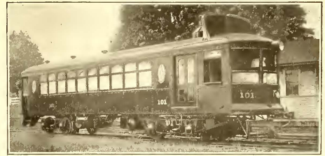
NEW TYPE OF STEAM-DRIVEN RAILWAY CAR USING GASOLINE OR KEROSENE AS FUEL
