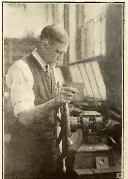
Fig. 6—Making a Core Loss Test. Fig. 7—An Impact Test on a Small Sample. Fig. 8—Subjecting a Sample to a Hammer Test. Fig. 9—Testing a Sample of Sheet Steel for Permeability. Fig. 10—The Draw Test of a Sample of Sheet Steel.
