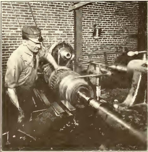
AT LEFT, SLOTTING A COMMUTATOR IN A DOUBLE-SPINDLE LATHE; AT RIGHT, REAR VIEW OF THE APPARATUS USED FOR COMMUTATOR SLOTTING
