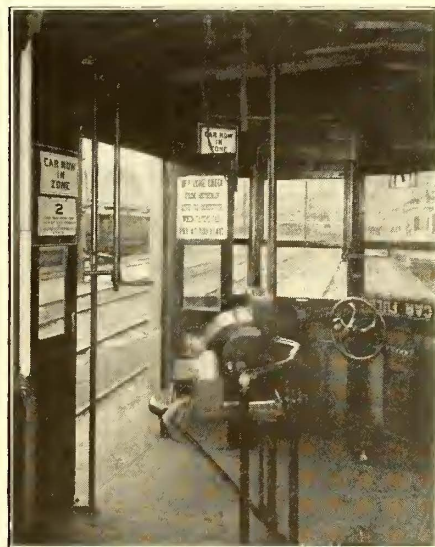
ARRANGEMENT OF REAR VESTIBULE SHOWING CASH REGISTER AND ZONE INDICATOR
