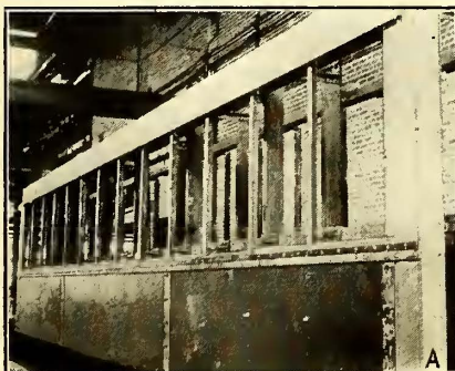
A—DETAILS OF SIDE CONSTRUCTION ON THE TEMPLATE WITH RIVETING PARTLY COMPLETED. B—METHOD OF ASSEMBLING SIDE FRAMES ON BODY BOLSTERS. C—THE FLOOR CONSTRUCTION INCLUDES SOME SPECIALLY DESIGNED MEMBERS
