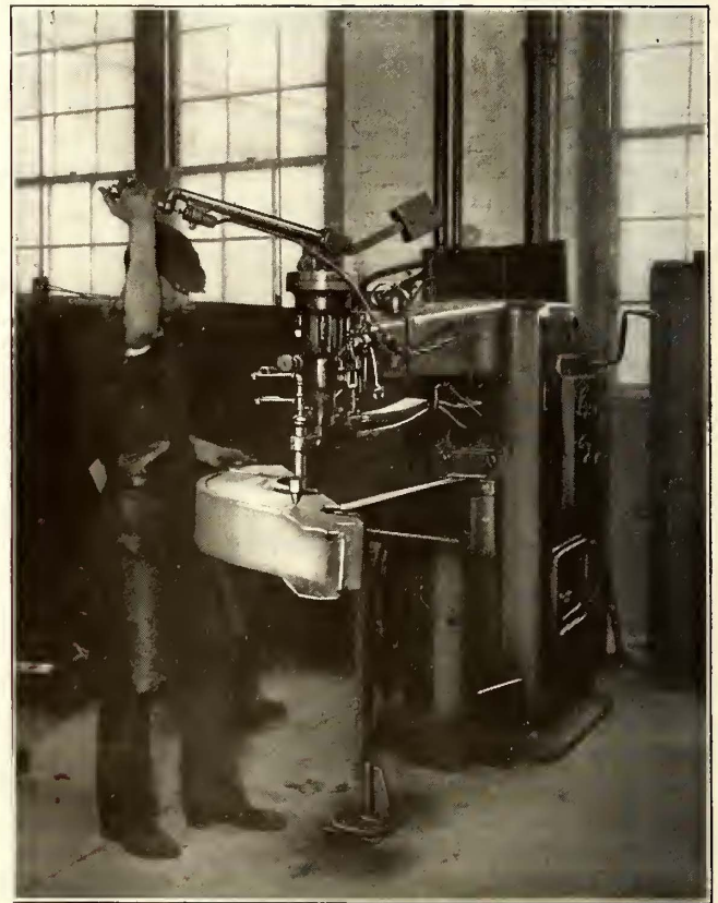
SPOT WELDING REINFORCEMENT TO GEAR CASE
