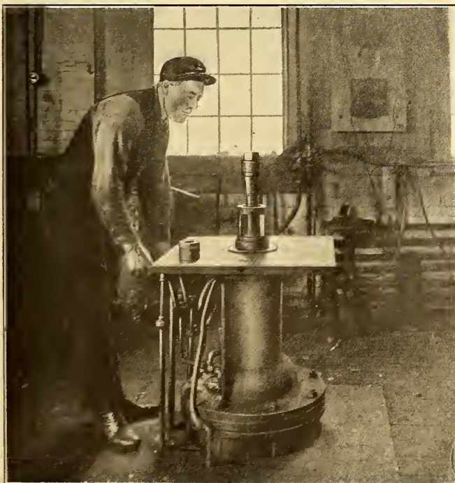
ALL BEARINGS WHICH ARE BABBITTED ARE BROACHED RATHER THAN BORED
