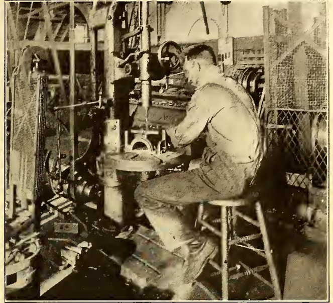
THIS JIG MAKES IT POSSIBLE TO DRILL ABOUT FORTY AXLE BEARING HALVES AN HOUR
