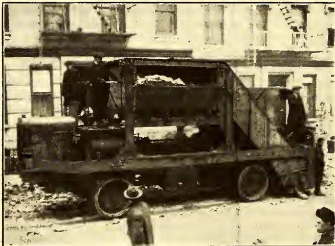
AT LEFT, ON DEMONSTRATION THIS SNOW "TANK" LOADED FIVE TRUCKS IN THREE MINUTES. AT RIGHT, THE "TANK" DIGS INTO A SNOW BANK WITH SHOVELS ON AN ENDLESS CHAIN CONVEYOR
