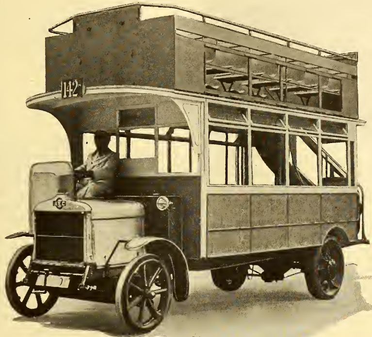
LONDON'S NEW DOUBLE-DECK FORTY-SIX-SEATER, WHICH WEIGHS ONLY 170 LB. PER SEAT
