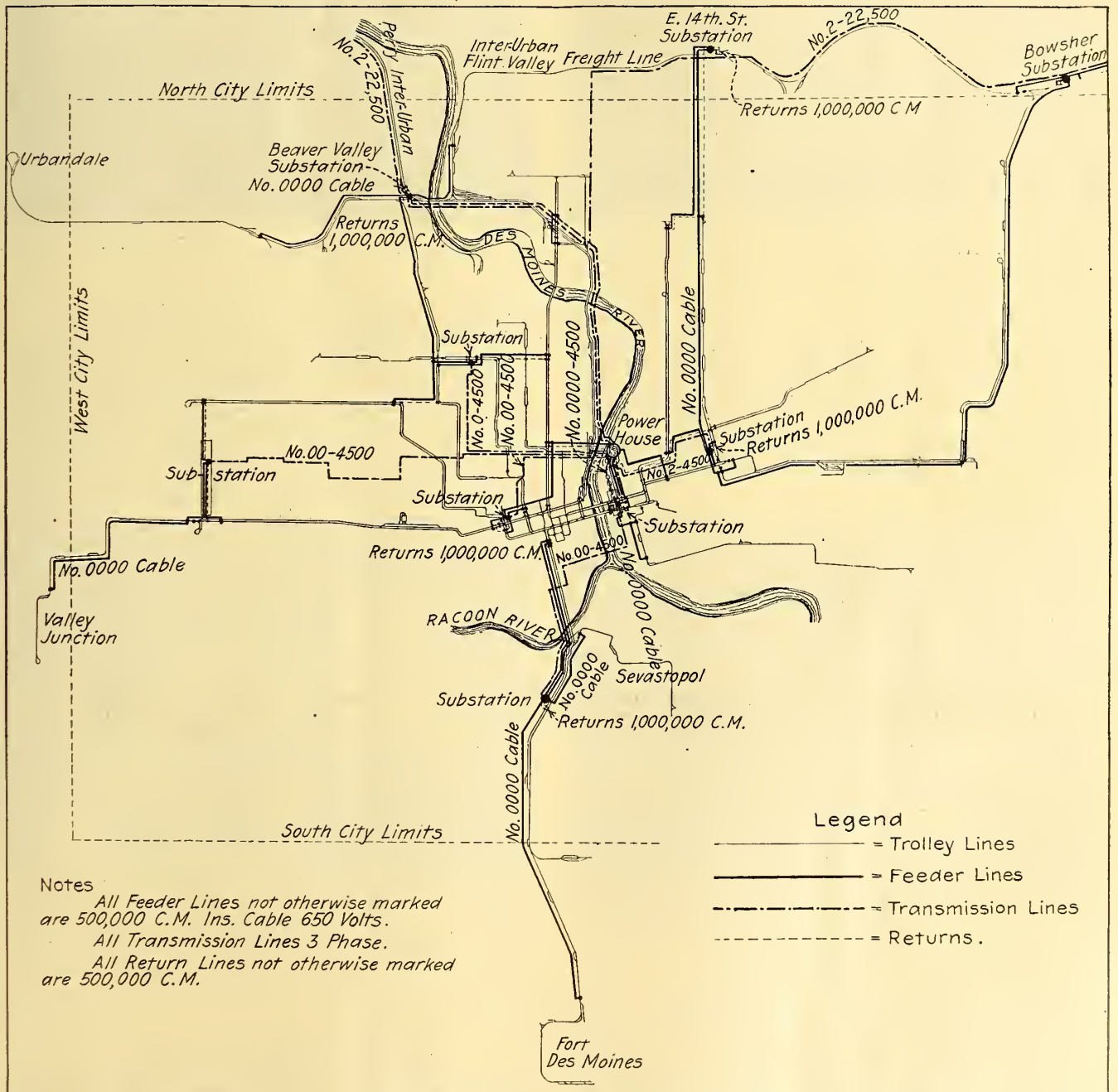
FIG. 3—OVERHEAD SYSTEM SHOWING FEEDER AND RETURN SYSTEMS AS ACTUALLY INSTALLED AND NOW IN OPERATION WITH SEVEN AUTOMATIC SUBSTATIONS. TOTAL AMOUNT OF COPPER, 460,000 LB. PRESENT TRANSMISSION LINE SYSTEM IS ALSO INDICATED
