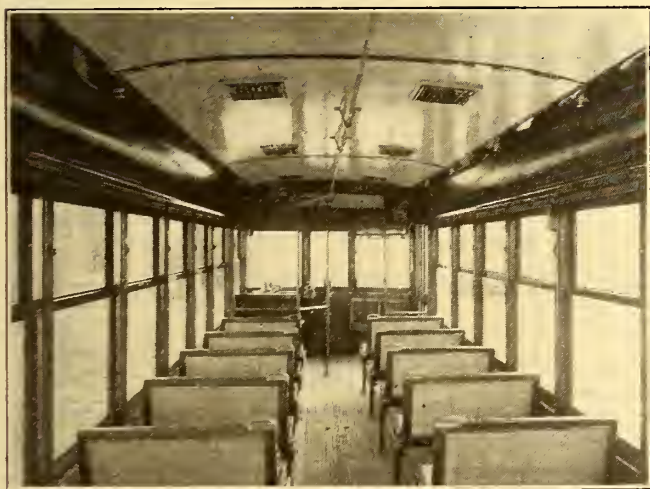
HEAD LINING, SIDE SHEATHING AND DOUBLE FLOORING WERE USED IN THE WAUKEGAN SAFETY CARS
