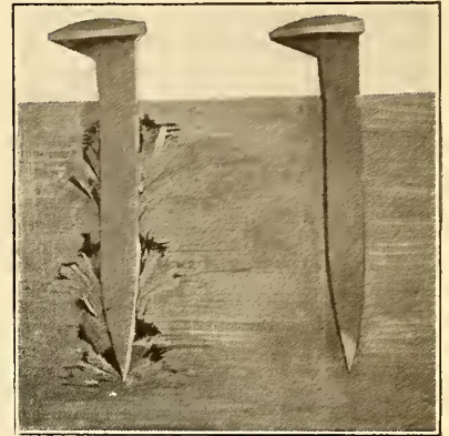
SECTION OF TIE WITH DRIVEN SPIKES
