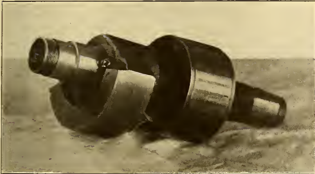
THE ROTOR AND UNBALANCED WEIGHT ON THE TAMPER MOTOR SHAFT
