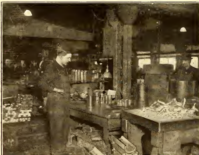
CORRECT METHOD OF HOLDING AND STEADYING THE LADLE WHILE POURING BABBITT INTO BEARINGS
