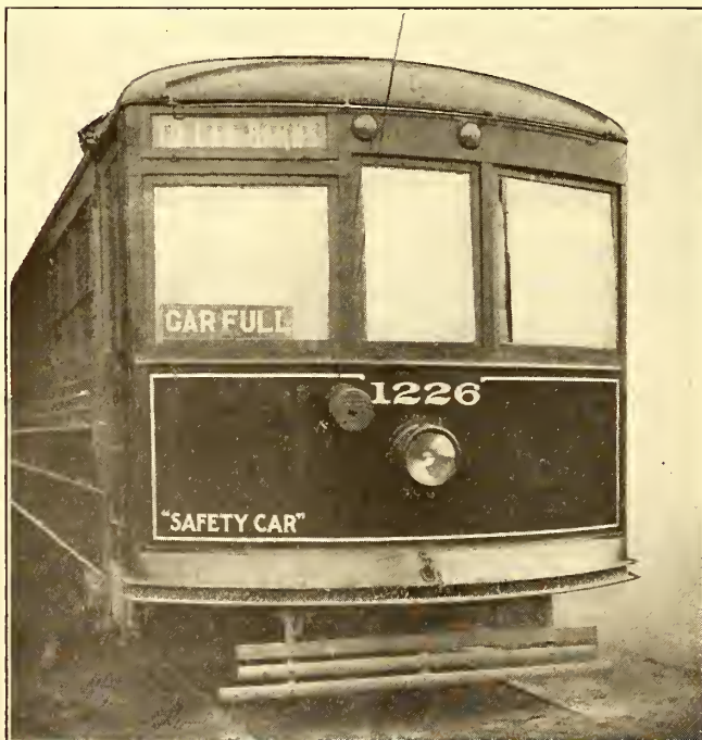
AT LEFT, "CAR FULL" SIGN USED ON RICHMOND (VA.) SAFETY CARS. AT RIGHT, THE REVERSE SIDE OF THE "CAR FULL" SIGN MAY BE SEEN IN THE RIGHT-HAND VESTIBULE WINDOW
