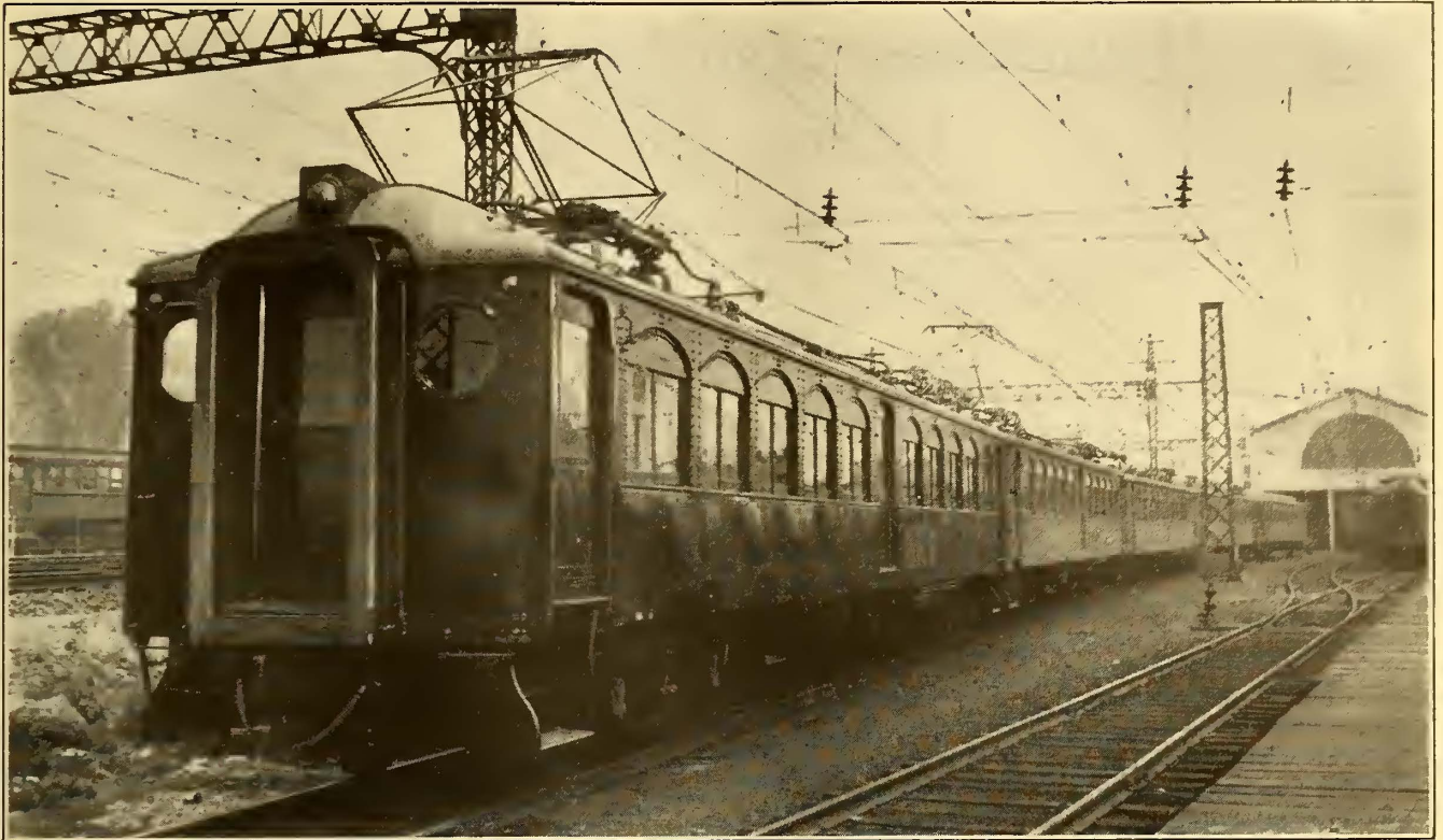
TYPICAL FOUR-MOTOR CAR TRAIN READY FOR RUSH HOUR SERVICE
