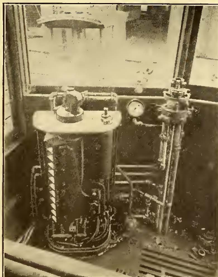
AT LEFT, PIPING TO BRAKE VALVE AND FOOT VALVE. IN CENTER, BRINGING PIPING BACK OF CONTROLLER. AT RIGHT, DOOR AND STEP CONTROLLER INSTALLATION
