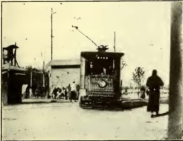
ONLY ONE TROLLEY POLE USED ON SHANGHAI RAIL-LESS BUS
