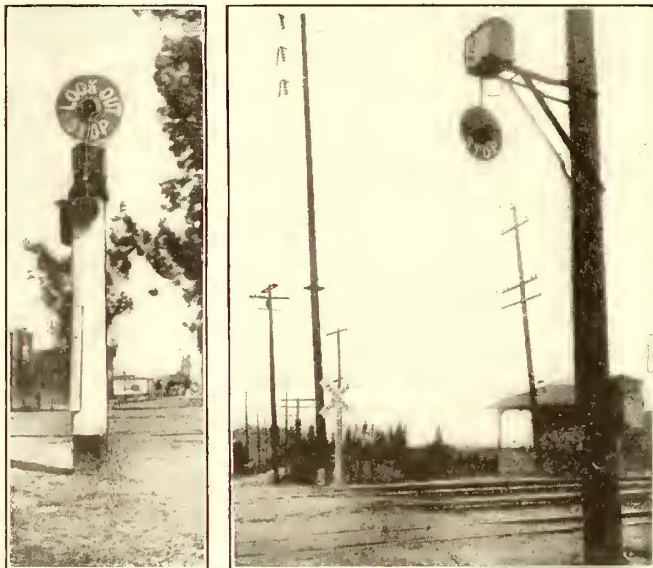
AT LEFT, SUPERSEDED TYPE OF MAGNETIC-AUTOMATIC FLAGMAN. AT RIGHT, LATEST IMPROVED TYPE OF AUTOMATIC FLAGMAN USED ON THE PACIFIC ELECTRIC RAILWAY
