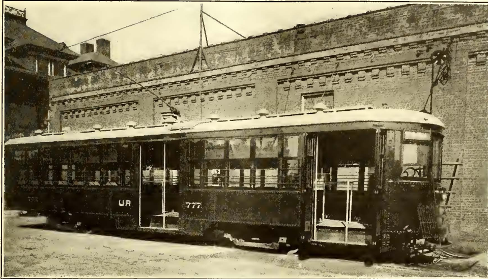
NEW PETER WITT TYPE MOTOR CAR FOR ST. LOUIS, HAVING ONLY TWO STEPS
