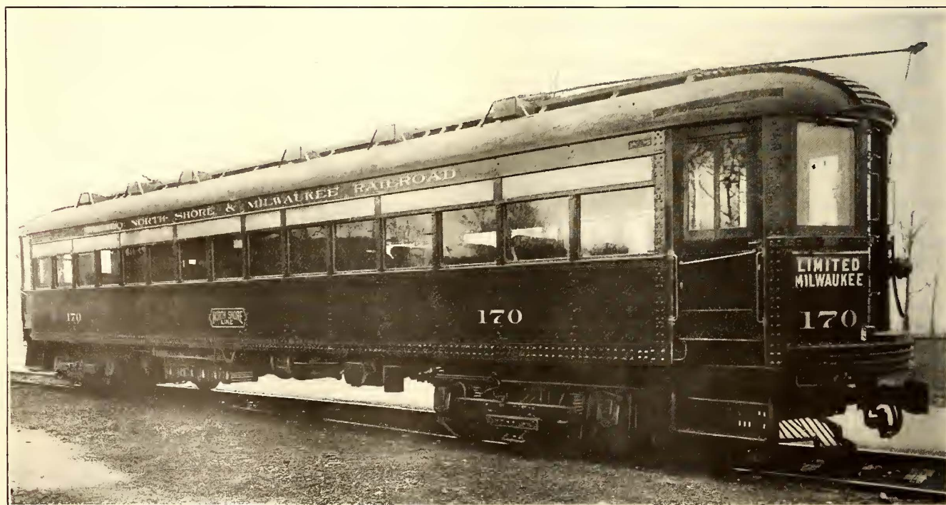
All-steel car designed to give the speed that has been an attractive feature of the North Shore service
