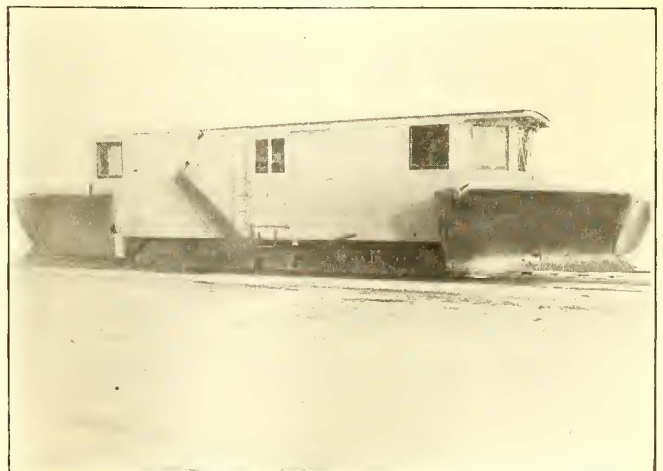
THE SHEAR PLOW IS USED ON DOUBLE-TRACK RIGHT OF WAY
