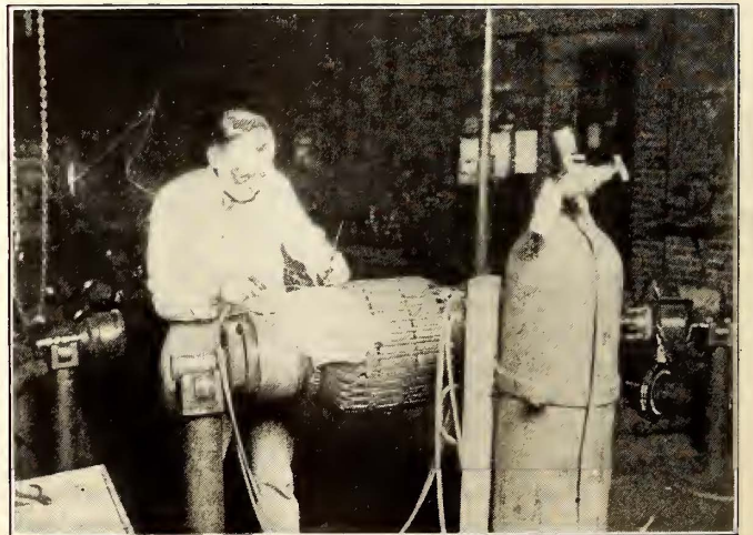
FIG. 5—GAS-WELDING BROKEN ARMATURE LEADS
