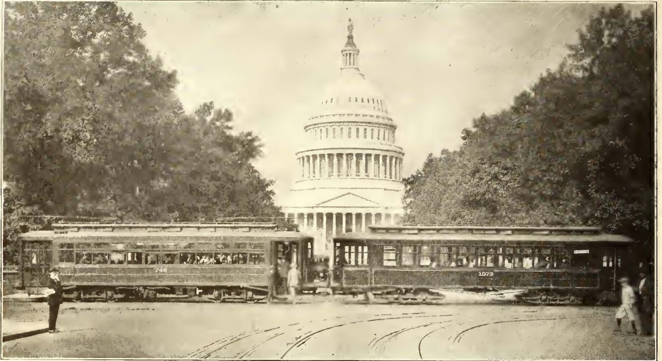
NEWLY CONSTRUCTED TRAILER COUPLED TO MOTOR CAR IN OPERATION
