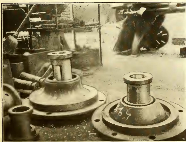
AT LEFT, BOX-TYPE MOTOR BEARINGS HAVE BEEN BUILT UP BY WELDING ON COPPER. AT RIGHT, A SPECIAL TRACKWORK JIG WHICH HAS GIVEN A GOOD ACCOUNT OF ITSELF
