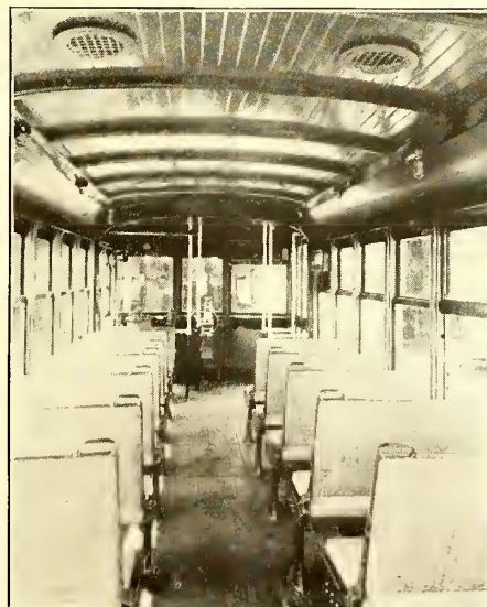
AT LEFT AND RIGHT, FRONT PLATFORM LAYOUT, SHOWING THE ARRANGEMENT OF STANCHIONS AND POSITION OF OPERATOR RELATIVE TO EXIT PASSAGEWAY. IN CENTER, INTERIOR OF MADISON CAR, SHOWING ABSENCE OF FOLDING PLATFORM SEATS, CURTAINS AND OTHER MOVABLE FIXTURES
