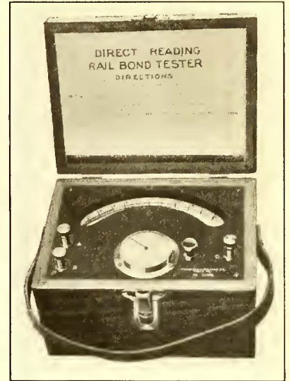
AT LEFT, PORTABLE STORAGE BATTERY EQUIPMENT FOR USE WITH BOND TESTER; CENTER, INSTRUMENT WITH SELF-WINDING TAPE AND MILLIVOLTMETER; AT RIGHT, DIRECT READING RAIL BOND TESTER
