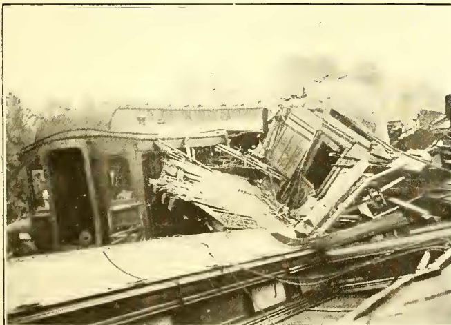
WHEN THE UNDERFRAME OF ONE CAR OVER-RIDES ITS NEIGHBOR THE UNDERFRAME ACTS AS A SHEAR AND SPLITS THE SUPERSTRUCTURE OF THE INVADDED CAR. THIS DERAILMENT OCCURRED AT A SPEED OF ABOUT 50 M.P.H.
