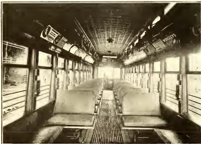
INTERIOR OF A CAR WITH VENDING MACHINES PLACED ON WINDOW POSTS
