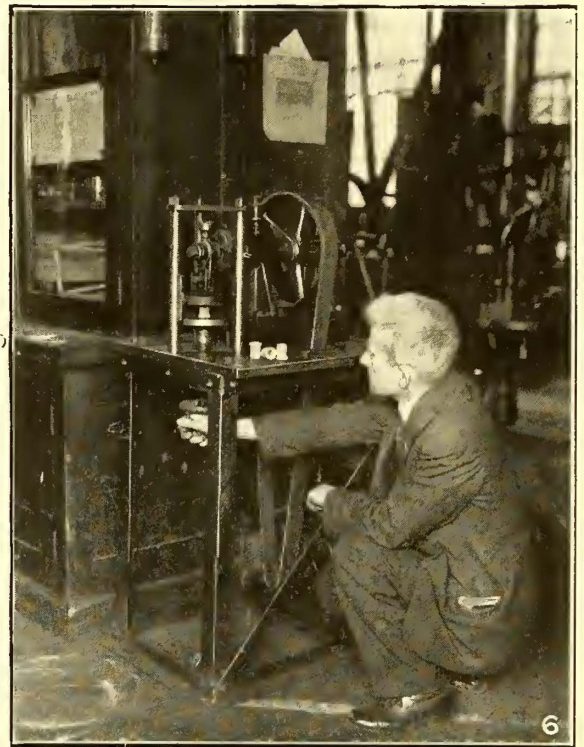
No. 4—Insulating gums are tested to determine the softening at different temperatures. No. 5—Viscosity of insulating varnishes is determined by a viscosimeter. No. 6—Rubber bushings are tested to destruction.
