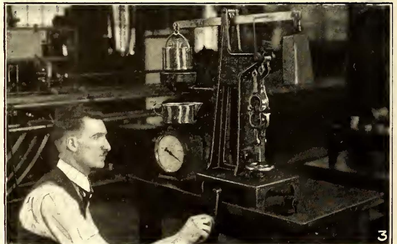
No. 1—Apparatus used in making tensile tests on tapes, cloths and cords. No. 2—Apparatus used in making rupture tests on papers. No. 3—This apparatus is used in testing the strength of cements.
