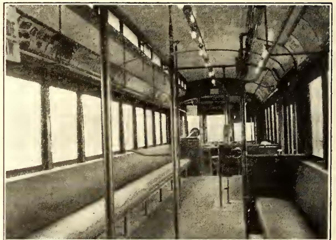
FIG. 3—INTERIOR OF THE FIRST CAR REMODELED FROM TRAILER TO FRONT-ENTRANCE, CENTER-EXIT TYPE
