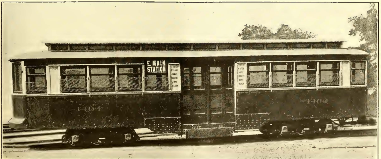
FIG. 6—THE FINISHED CENTER-ENTRANCE TRAILER MADE FROM A CENTER-ENTRANCE MOTOR CAR
