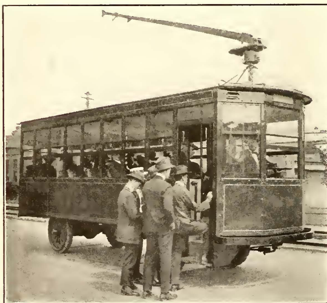
GENERAL VIEW OF TROLLEY BUS, MOUNTED ON SOLID RUBBER CATERPILLAR TIRES
