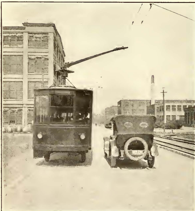
AT LEFT, NO DIFFICULTY IS EXPERIENCED IN PASSING VEHICLES ON THE ROADWAY; AT RIGHT, TROLLIBUS TAKING 90-DEG. CURVE. NOTE THE SYSTEM OF OVERHEAD TROLLEY CONSTRUCTION
