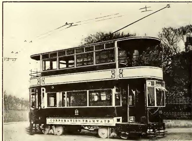
SAMPLE REBUILT DOUBLE-DECK CAR, SHOWING VESTIBULING AND OPEN PORTIONS OF UPPER DECK
