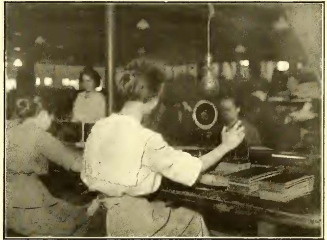
MICA FOR RAILWAY MOTOR COMMUTATORS IS TESTED FOR UNIFORM THICKNESS
