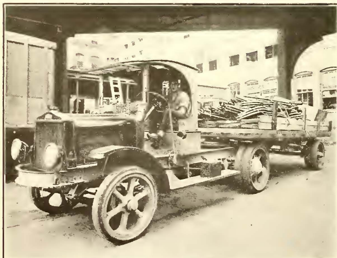
TYPES OF TRACTOR AND TRAILERS USED TO HAUL MERCHANDISE BETWEEN RAIL TERMINAL AND DOWNTOWN STATION— NOTE TRAILER SUPPORTS FOLDED BACK FOR CLEARANCE ON ROAD
