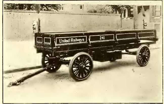
THIS TRAILMOBILE IS USED TO CARRY HOSE BRIDGES
