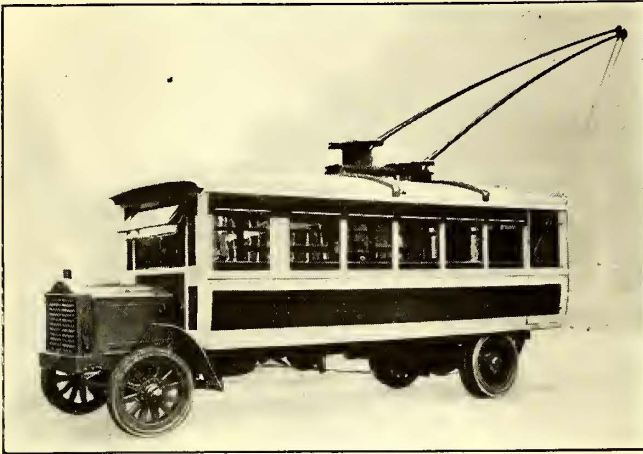
PACKARD TROLLEY BUS COMPLETE WITH THE STANDARD GAS-ENGINE CHASSIS
