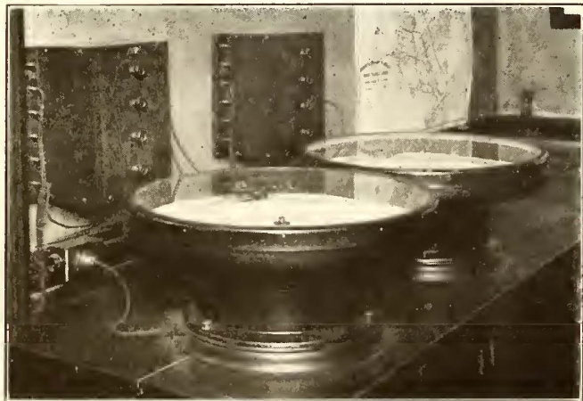
TWO HEDWAYGRAPHS ARE LOCATED IN THE CHIEF DISPATCHER'S OFFICE
