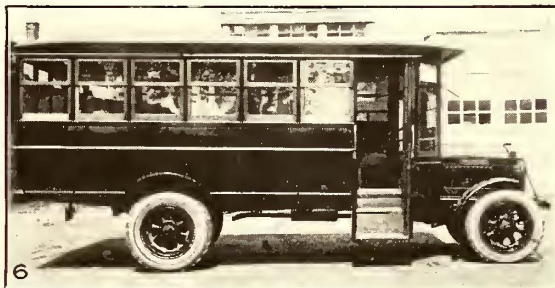
Fig. 1—The Ultimate Truck, Type AJL. Designed and built by Vreeland Motor Company, Inc., Newark, N. J. Seating capacity twenty-two. Uses Buda motor with Sheldon worm drive.
