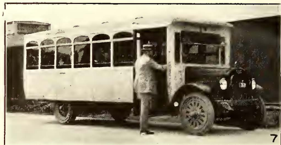
Fig. 5—The Imperial Omnibus. Designed and built by the Trackless Transportation Company, New York. A low center of gravity type omnibus. Buda motor and Clark type rear wheel internal drive. Kuhlman truss side all steel body. Seating capacity twenty-nine.
