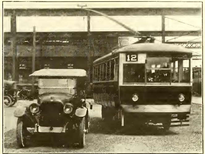
"Rail-less" Car Developed by J. G. Brill Company, Philadelphia, Pa. Seating Capacity Twenty-eight. General Electric Equipment Used
