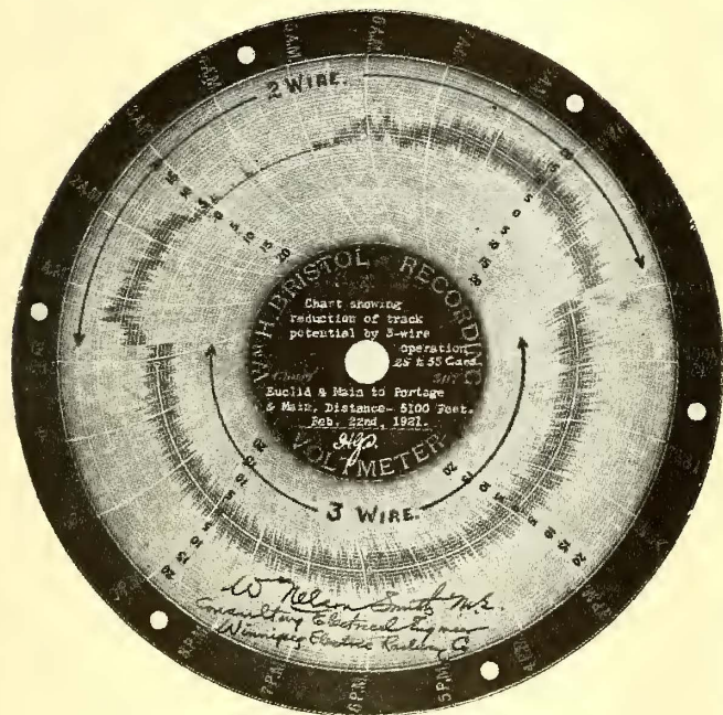
TRACK POTENTIAL ON MILE SECTION IN WINNIPEG, USING TWO-WIRE AND THREE-WIRE SYSTEM
