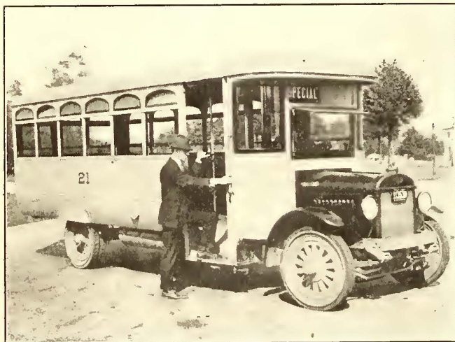
THE NEW BALTIMORE BUS, WITH ITS SINGLE 15-IN. STEP AND 26-IN. SERVICE DOOR, IS CONVENIENT TO BOARD
