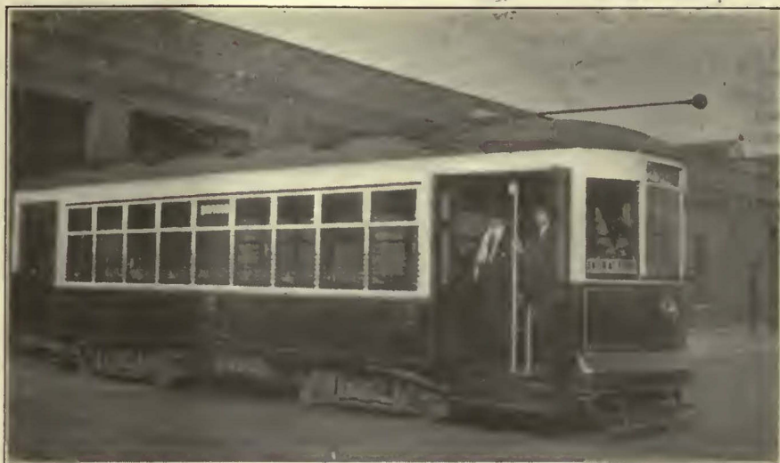
THE 37-FT., 45-PASSENGER DOUBLE-TRUCK ONE-MAN CAR NOW BEING TESTED BY THE CHICAGO SURFACE LINES
