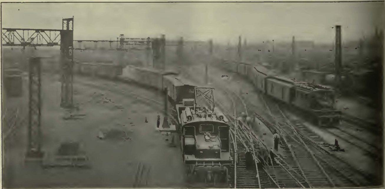
CLASSIFICATION AND SWITCHING SERVICE IS EASY WORK FOR THESE LOCOMOTIVES, WHICH HAVE A TRACTIVE EFFORT OF 23,200 LB. AND A RATING OF 752 HP.
