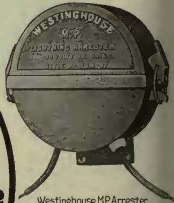
Westinghouse MP Arrester 400-750 Volts A-C, or D-C, Style 154,297
