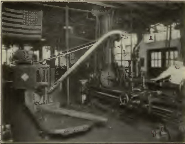
CRANE TRUCK SERVING SHOP MACHINE
