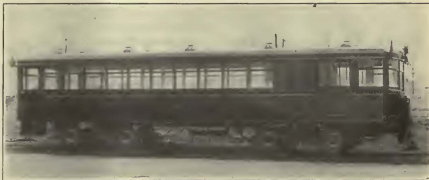
GASOLINE CAR FOR RAIL SERVICE. IT WEIGHS 13 TONS AND CARRIES THIRTY-EIGHT PASSENGERS, WITH DROP SEATS FOR EIGHT IN BAGGAGE COMPARTMENT
