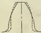
"Safety Car" Type 12 teeth, 4\frac{1}{4} pitch, WISDOM-TOOTH contrasted with 13 teeth, 4\frac{1}{4} pitch, standard tooth.
