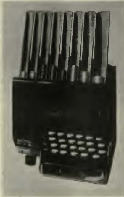
LEFT, TICKET-ISSUING CASH REGISTER AND, CENTER, CILANOE-MAKER IN WABASH AVENUE STATION, CHICAGO. RIGHT, SAMPLE TICKET —AR DESTINATION "2" SHOWN IS NUMBER OF ISSUING STATION AND NO PRICE IS PRINTED. THE TICKET IS NOT GOOD FOR TRANSPORTATION
