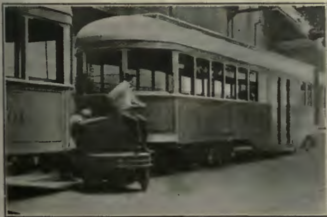
SWITCHING CARS IN THE SHOPS OF THE CLEVELAND RAILWAY. THERE IS EVEN ROOM FOR THE TRACTOR TO MANEUVER BETWEEN THE TWO CARS BEING COUPLED
