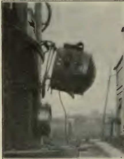
MECHANISM FOR TILTING ARC HEADLIGHTS ON INTERURBAN CARS, AND, AT RIGHT, LEVER AND CONNECTING MECHANISM FOR TILTING HEADLIGHTS
