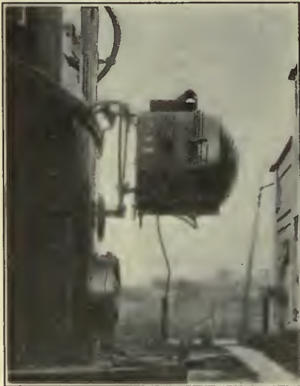
MECHANISM FOR TILTING ARC HEADLIGHTS ON INTERURBAN CARS, AND, AT RIGHT, LEVER AND CONNECTING MECHANISM FOR TILTING HEADLIGHTS
