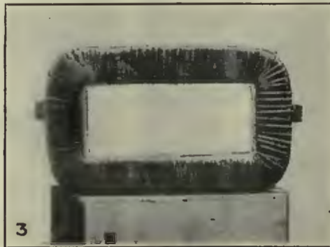
NO. 1—METAL FIELD SHELL AS ORIGINALLY USED. NO. 2—FIELD SHELL SAWED IN TWO PIECES AS USED WITH NEW FIELD COIL. NO. 3—FORM-WOUND FIELD COIL READY FOR INSTALLATION. NO. 4—WINDING FORM FOR USE WITH NEW TYPE FIELD COIL
