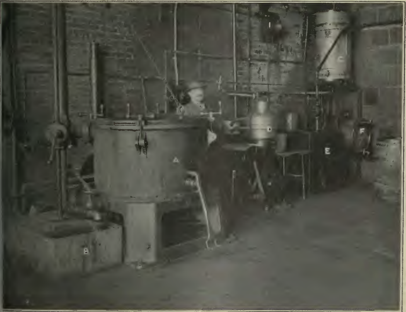
INTERIOR OF OIL HOUSE, SHOWING ARRANGEMENT OF EQUIPMENT USED IN OIL EXTRACTION AND IN WASTE RECLAMATION
