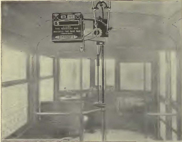
A one-man car equipped with an Ohmer Fare Register with a capacity of twelve different fare classifications.
