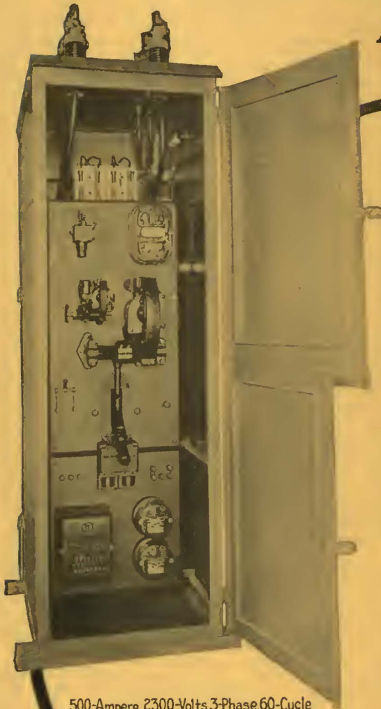
500-Ampere, 2300-Volts, 3-Phase, 60-Cycle Automatic Outdoor Switch House, Periodic Re-closing Feeder Equipment.—Front View.
