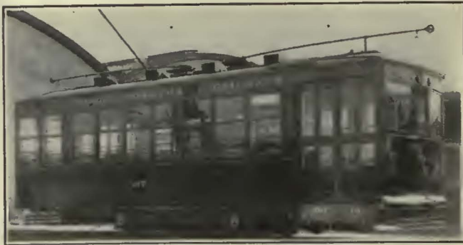
DOUBLE-DOOR OPENINGS ARE A FEATURE OF THE HYDRO-ELECTRIC CARS
